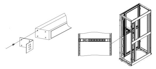
Vertically mounting(any standard 19-inch EIA/ECA-310 rack or enclosure, applied in horizontal units) 1.Attach the vertical-mounting brackets to the PDU.
